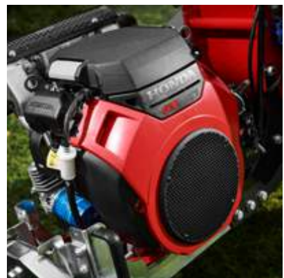
2-cylinder air-cooled HONDA petrol engine with electronic ignition
