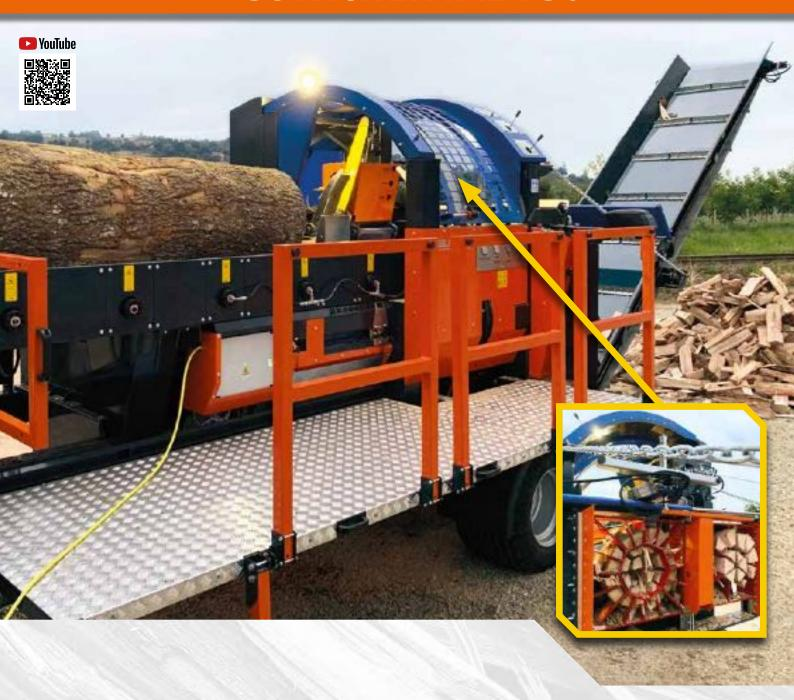
Balfor's Continental 750 Special ranks among the largest high productivity firewood processors on the market. With the ability of cutting up-to 70cm in diameter and with a splitting force of 50 tons, it is able to perform in all situations.
