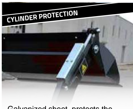
Galvanized sheet, protects the moving parts from materials that could damage them
