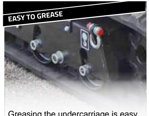
Greasing the undercarriage is easy and fast: nothing has to be taken apart.
