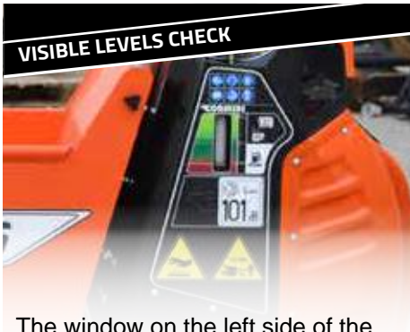
The window on the left side of the unit allow an immediate check of the fuel level
