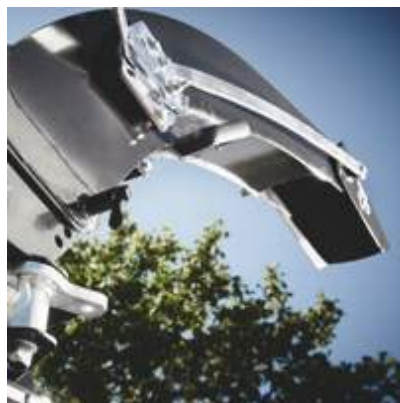
TP VARIO SPOUT. Adjustable height with 5 out-put positions
