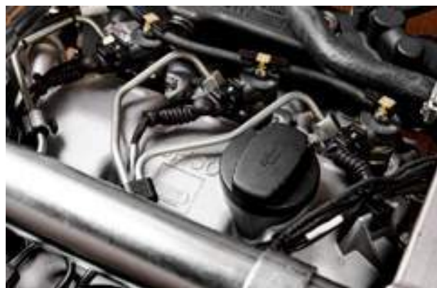
Hatz engine from Germany, Stage V with Bosch common rail system
