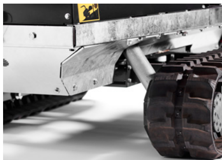
Ground clearance of 220 mm, easy service and reinforced hose protection. Variable track width 1000-1400 mm
